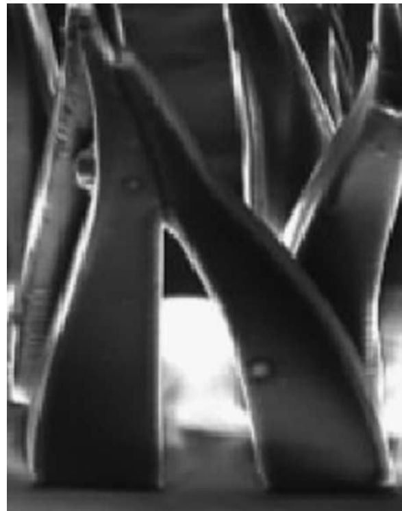
Figure 3. Typical clumping behaviour observed between adjacent stalks for very soft materials such as Silicones Inc. P-20. Stiffer materials did not exhibit extensive clumping.
