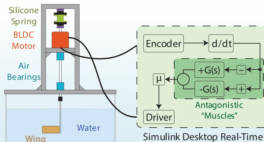
We built a **dynamically-scaled spring-wing system** (detailed in [4]) of a flapping insect consisting of
