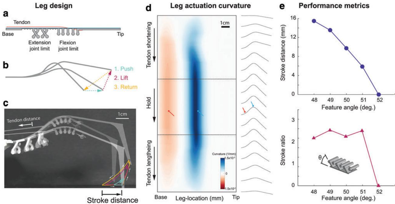
measuring the limb curvature and shape change (Fig. 5d) and stroke properties (Fig. 5e). Tracking the continuous curvature of the limb during the actuation cycle highlights how flexoskeleton limbs behave as a continuum structure with a gradient in shape and curvature (Fig. 5d). This is in stark contrast to more traditional link-joint limb designs in which the curvature would be observed as a delta function at each joint.
