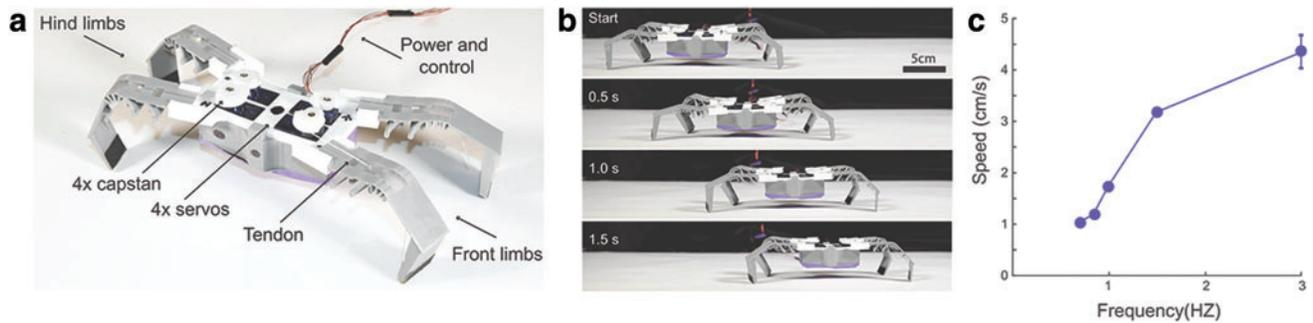
**FIG. 6.** A walking quadruped flexoskeleton robot. **(a)** Each limb is actuated by a single servo and tendon. Off-board power and control are provided through a tether. **(b)** A side view of a walking sequence. **(c)** Speed–frequency relationship of the walking performance of the robot. Color images are available online.
