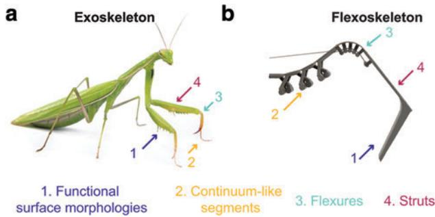
**FIG. 1.** (a) The exoskeleton of an insect provides protection and serves to support locomotion through structural and flexural regions. (b) In this article, we introduce a new method for fabricating exoskeleton-inspired robots that seek to embody the four principles of the exoskeleton. Color images are available online.
