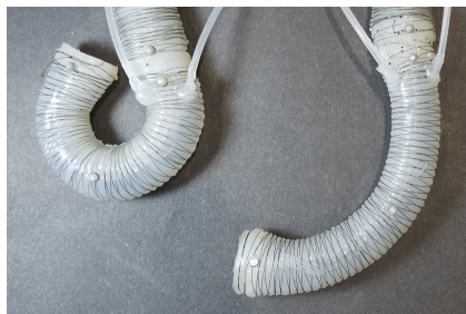
Fig. 1: Inextensible (left) vs. extensible (right) backbone curvature at 0.02 MPa
